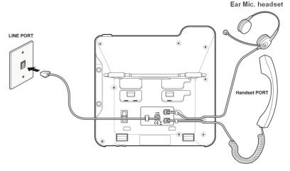
Figure 5 Edge 9200 series Connections
